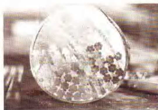
Fig. 19.2 Tendon Slice Showing Penetration of Grout Between Strands 19.12
