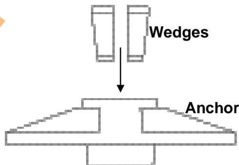
Figure 3.4 Wedges insert into anchor
