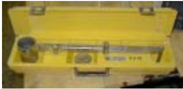
Fig. 9: Mud Balance equipment for density measurement of fluid grout.
